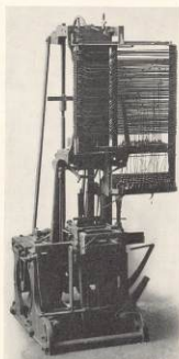
FIG. 3.—Mergenthaler's second "band" machine of 1884, on which the first line-of-type was cast, and in which a casting apparatus was first used, reproduced from a photograph of an incomplete and damaged machine, the last survivor. See description under Fig. 4.
