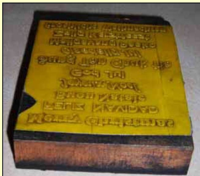
10 Above is a finished plate fixed to a wooden mount. The plate has been used and was lightly cleaned so that the image would be visible. The plate is fixed to the mount with double-sided carpet tape. The plate and mount are type high.
