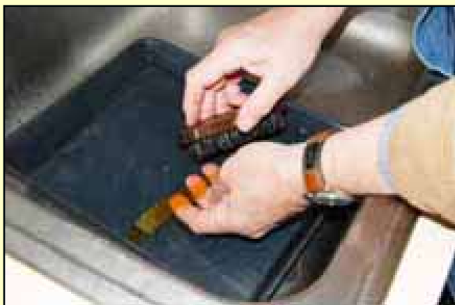
9 The raised image can be felt and seen as the unexposed polymer is removed. The plate is ready when only the image and the clear plastic backing can be seen. (Photo by Bradley)
