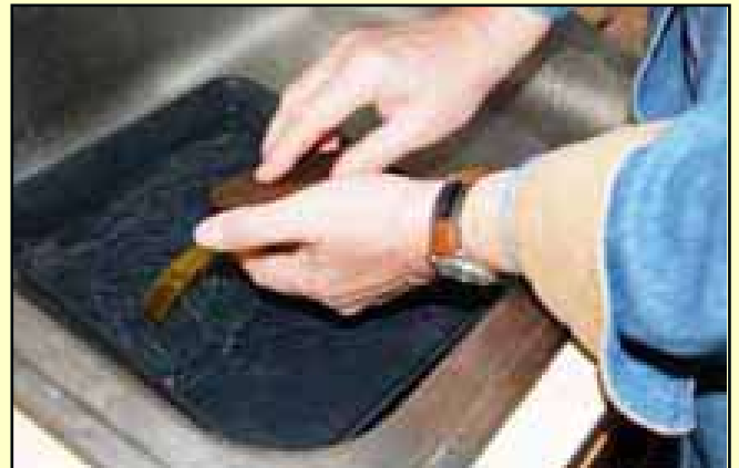
8 The exposed photopolymer plate is emerged in warm water and lightly scrubbed until all the unexposed polymer is removed. (Photo by Bradley)
