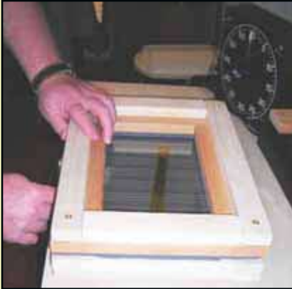
5 The contact box top is closed and locked over the guide and photopolymer, sandwiching them between the two pieces of glass.
