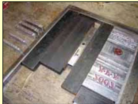
Cover locked up and ready for the press.
