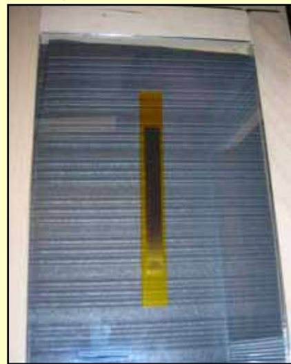
4 A Stouffer Scale 21 Step Sensitivity Guide is placed on top of a strip of photopolymer to determine correct exposure time with the photopolymer and the UV lights.
