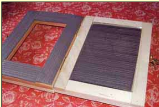
2: Contact box with lid open, showing the bottom frame with carpet padding inserted and fixed to parameter of top frame.
