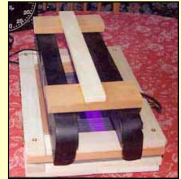
4: Completed contact box with UV showing details of UV lights joined with I-beam.
