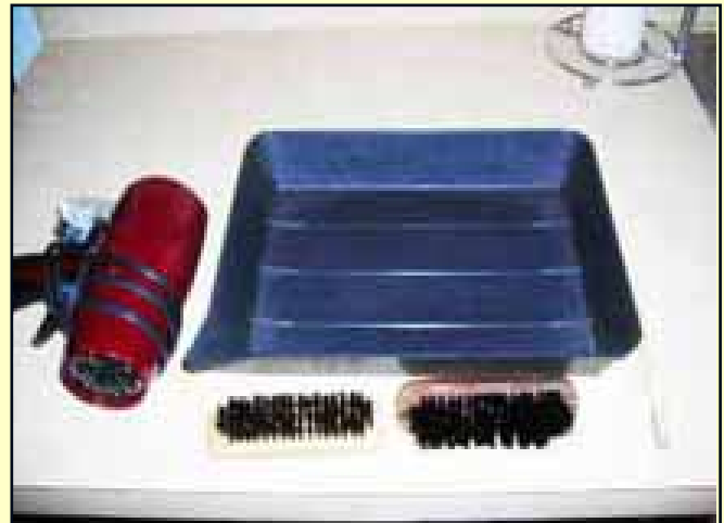
7 Above are the items required to complete the development of the photopolymer plates: hairdryer, washout tray, Kiwi shoeshine brushes and toothbrush are shown.
