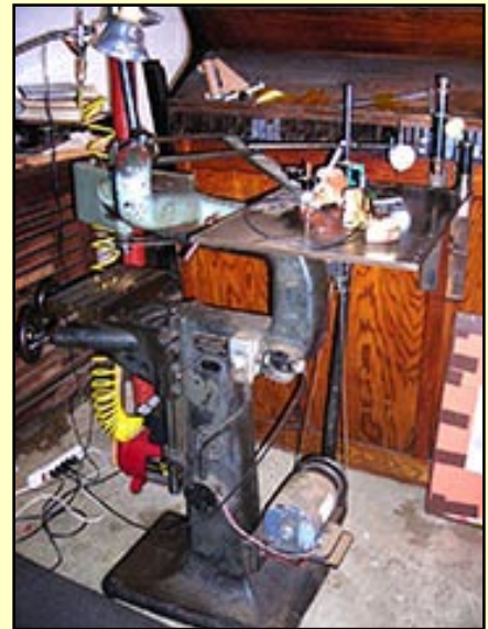
The Deckel Engraving machine (above) that is used in making matrices. The Pattern Board is on the right holding tool used in the making of matrices. The Engraving Board is to the lower left. The Air Compressor, used to remove chips, can be seen on the floor.
