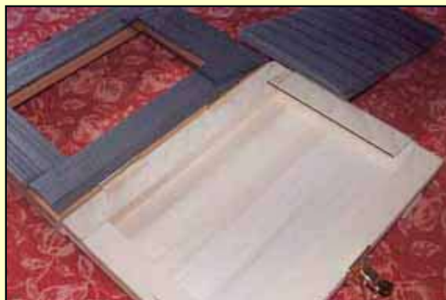
3: Contact box open showing construction of bottom frame without carpet.
