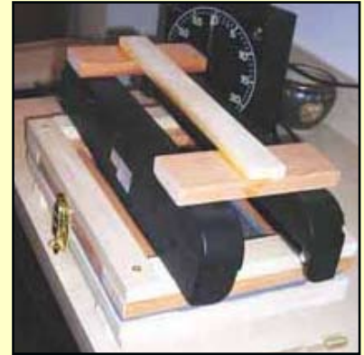
3 Above is the contact box with two UV lights connected by a wooden I-beam on top.
