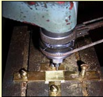
A close up of the Cutting Arm of the Deckel Pantograph shows the quill with cutting tool positioned on a blank matrix. Once the cutter has been properly positioned, the Cutting Board will be raised .015" and the cutter lowered into cutting position.
