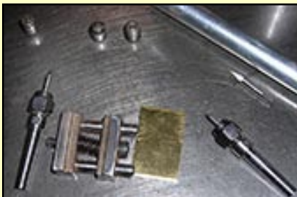
Above are shown two quills with different size cutters inserted, the mini-vice and a blank matrix. Top are three different followers, the main body, or button, fits on the end of a brass rod on the Follower Arm of the Pantograph, the follower itself is the needle like projection in the center. The smallest of these three followers (right) measures .00135". Also shown is a 1/4" Cutter and the 40x Mini-Mike.
