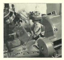
11. Turn the machine to 20°. If the 1—3 point mould is to be used, attach the special blade connection (29) which is stored in the mould box, to the mould blade slide with the pin (turning clockwise until it grips) and tighten the set screw (30).
