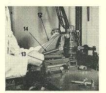
6. Remove the Composition matrix head (12) from the matrix heads base (13), by disconnecting the matrix lifter connecting rod (14) from the matrix cam lever, and removing the three short screws and one long screw.
