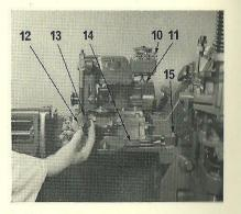
4. Take off the mould oiler piping and support, by first setting the valve lifters (10) in the horizontal position, and then loosening the knurled nut (11).
