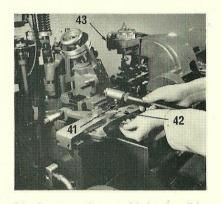
16. Connect the mould blade slide drive lever connecting rod ball end (41) to the intermediate lever (42) in the position marked *Furniture*, seating the snug pin in the groove, and securing with the nut. Place the 3 em setting gauge between the fusing stop and the lower edge of the blade, adjusting the wedge until it is lightly held. Set the scales on the wedge screw handwheel to zero.
