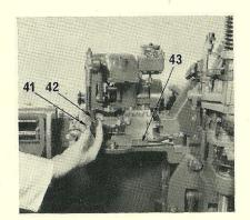
13. Connect the lead clamp intermediate lever rod yoke (41) to the lead clamp lever with the pin. Replace the clip (42) over the pin to secure in position.
