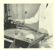
9. Attach the lead stacker bar (31) to the lead stacker (32), with the two screws and washers already in position on the stacker.
