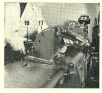
8. Disconnect the rod yoke from the type carrier cam lever extension by removing the screw and position pin.
