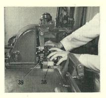
12. Turn the machine to 200° and place the mould blade slide in the backward position. Place the furniture mould (38) on the main stand and push the jetblock carefully out of the mould until the hook is clear. Slide the mould into position so that the hooks (39) engage.
