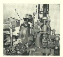
2. At the same time, set the trip plates (5) and stop plates - known as upper and lower leaves - for the required product: adjust the piston spring rod nut, and check the nozzle seating timing device (6). The timing device, as a general rule, is used whenever the 14" pump is in operation, together with the No. 5 nozzle and speeds from 4½ to 12 r.p.m.
