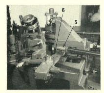
2. Disconnect the mould blade slide drive lever connecting tube ball end (5) from the intermediate lever (6), by removing the nut. Lift the lever out of engagement and pivot to one side, replacing the nut on the ball end to avoid loss.
