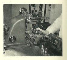
4. Turn the machine to 20°, raise the stop lever handle (18) to its highest position (see picture 5) and remove the product from the mould. Place the mould blade slide in its forward position to clear the blade connection from the wedge screw housing base, or with the 4—18 point mould, to disconnect the mould blade from the slide. Remove the four screws securing the mould to the main stand, and then the clamps from the side and the front.
