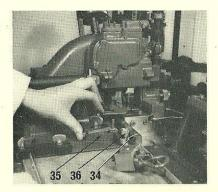
14. Check that the fixed type channel block (34) is correct for the product to be cast, and change if necessary.
