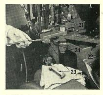
8. With the stop lever handle (21) in the low position marked *Leads*, turn the plunger spring adjusting nut anticlockwise so that the spring will exert only minimum pressure. Set the fulcrum pin at the 1—3 L and R position.
