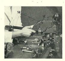
5. Remove the four screws securing the display matrix head (14) to the base. Take a firm grip on the head and lift it off the machine.
