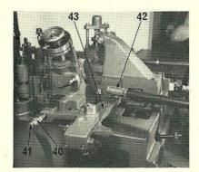
15. Check that the driving block cap abutment (40) is correctly positioned, the large diameter end towards the front of the machine to produce type in set sizes 12 points and below. To reverse the abutment, remove the hexagonal screw (41).
