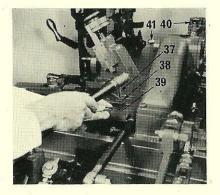
16. Connect the mould blade slide drive lever connecting tube ball end (37) to the required hole in the intermediate lever (38) for the set size to be cast. Seat the snug pin in the groove and secure with the nut (39).
