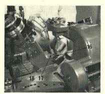
5. After removal of the 1—3 point mould, and with the blade connection (16) still clear of the wedge screw housing base, release the set screw (17) and remove the pin so that the blade connection can be taken off. Replace the pin in the mould blade slide, and tighten the set screw so that its head is below the top surface of the slide. This will prevent damage if the slide should be withdrawn.
