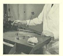
6. Take off the lead stacker bar (15) by removing two screws (16) and washers which hold it to the lead stacker. Replace the screws and washers in the bar to avoid loss. Release the lock screw to free the cutter actuating lever pin, and then remove the cutter blade. Take off also, the cutter blade bracket (17) (see picture 7), which is held by two screws, and the lead guide bracket.
