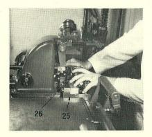
9. Turn the machine to 200° and place the mould blade slide in the backward position.
