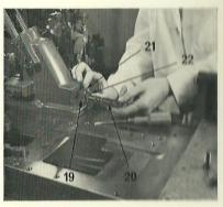
8. Bring the mould blade slide (19) forward to expose completely the mould blade fork (20). Free the connecting pin by a half turn anti-clockwise of the locking screw (21), and then remove the pin (22) to disengage the fork. It is important to ensure that the head of the lock screw is not left pretruding above the face of the mould blade slide, or it will be damaged when the slide is withdrawn.
