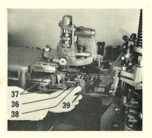
its adaptor base; place the low quad lever spring lever in the required position, and connect the spring plate (36) to the mould blade lever. Place the type clamp block in position and secure with its two screws.
