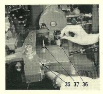
11. Turn the eccentric plunger lever fulcrum pin (35) to the 1-3 L and R position. Hang the weight (36) from the hook on the ratchet pin chain, and remove the pin (37) which connects the actuating rod to the housing.
