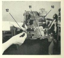
4. Remove the mould oiler piping and support from the underside of the mould oiler by releasing the knurled nut (10). Disconnect the mould water supply piping (11) from the mould, and loosen the nut on the main stand stud so that the piping can be pivoted aside.
