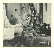
6. Disconnect the matrix lifter lever connecting rod yoke (15) from the cam lever by removing the nut and eye pin.
