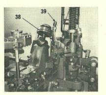
14. Engage the nozzle seating timing mechanism by lifting the release knob (39) and freeing the timing lever (38) with a flick of a finger.
