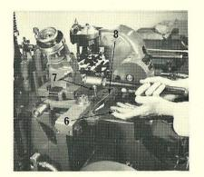
3. Unscrew the lock nut (6) and disconnect the mould blade slide drive lever connecting tube ball end (7) from the furniture position on the intermediate lever (8).
