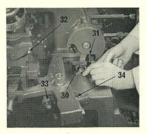
10. Disconnect the actuating rod eye from the rod housing, and re-connect it by its upper hole to the actuating lever (30) with the pin. Hang the weight on the hook of the ratchet pin chain (31).
