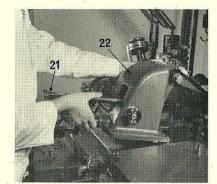
7. Disconnect the jet block driving rod connecting rod yoke from the type carrier cam lever extension by removing the screw and the yoke position pin. Replace the pin and screw in the yoke, after disconnection, to avoid loss.
