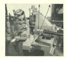
2. Disconnect the mould blade slide drive lever connecting tube ball end (3) from the intermediate lever (4), by removing the stud nut from the underside of the lever and lifting the ball end out of the hole. Move the tube to one side so that it is clear of the top of the machine.
