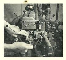
3. Remove the matrix holder (8) from the display matrix head, by pulling the small release lever with the fingers of the left hand, and withdrawing the holder with the right hand. After casting quotations, ensure that the matrix lifter handle is returned to its normal position by raising the lock pin knob on top of the matrix head.
