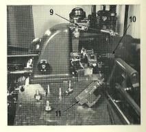
4. Remove the product from the mould, Disconnect the lead clamp intermediate lever rod (9) from the mould by removing the yoke pin, and pivoting upwards. Disengage the mould water supply piping (10), and take off the furniture guide (11) from the main stand.
