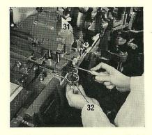
14. Cover the locating faces of the mould water supply piping (31) with grease, fasten one end to the main stand stud with the washer and nut, and the other end to the mould with the screw. Tighten the screw before the nut and washer.
