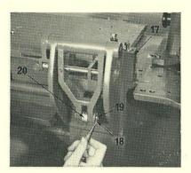
7. Disengage the cutter actuating lever from the cutter actuating plunger by first removing a split pin (18) from the link pin (19). The link pin can now be withdrawn sufficient to allow the actuating plunger (20) to drop free.
