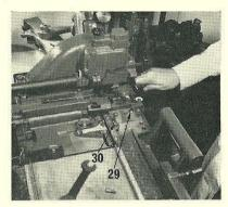
11. Place the mould blade slide in the forward position and attach the mould blade fork, of the required point size, with the pin. Turn the pin clockwise until it grips and then tighten the screw.
