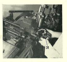
12. Connect the mould blade to the fork, inserting the pin with the aid of a pin handle. Draw back the mould blade, by turning the knurled nut, until the pin is contacted and then tighten the knurled lock nut.
