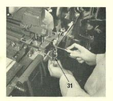
12. Select the mould oiler (31) suitable for the mould being used, and attach it to the mould.
