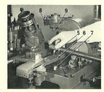
2. Disconnect the tube ball end (5) from the intermediate lever (6) by removing the nut (7) and lifting clear. Replace the nut on the tube ball end to avoid loss. Remove the mould oiler piping and support from the mould oiler (8), by placing the valve lifters in their horizontal positions and loosening the knurled nut (9). Remove the galley side wall from the galley plate.
