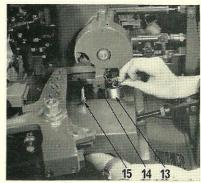
7. Unhook the weight (13) from the ratchet pin chain and lay it on the shelf inside the main stand, convenient for reconnection.
