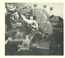
11. Attach the actuating lever link (31) by placing the elongated eye (32) over the pin on the actuating lever, and connecting the hook (33) at the other end to the fusing stop (34) on the mould.
