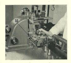
13. Support the mould on the main stand, and carefully push the jet block forward until the hook (32) is clear of the mould. Tilt the mould, so that the hooks can be positioned one over the other, and then slide the mould to connect the mould blade to the mould blade slide. Secure the mould to the main stand with the clamps at the front and side, and the four screws through the top of the mould.
