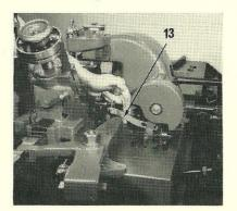
5. Take off the actuating lever link (13) by unhooking it from the fusing stop on the mould, and releasing the eye from the pin on the actuating lever.
