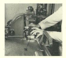
7. Turn the machine to 200° and pull back the fusing stop to place the mould blade slide in the forward position. Loosen the set screw in the slide and remove the pin to disconnect the blade from the blade slide.
