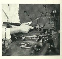
4. Withdraw the mould guard hinge pin and remove the guard (9) from the matrix head (10). Remove three screws securing the matrix head, and free the fourth screw (11) so that the matrix head may be lifted off.
