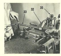
11. Attach the composition matrix head (32) to the matrix heads base and secure with three screws and the one long screw. Connect the matrix lifter lever connecting rod (33) to the top hole of the matrix cam lever (34) with the rod eye pin and nut.
