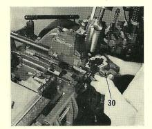
13. Connect the mould blade to the fork, inserting the pin with a pin handle. Turn the knurled nut until the mould blade contacts the pin, and then tighten the lock nut, using pin wrenches.
