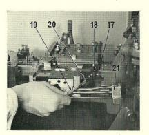
7. Release the knurled lock nut (17) on the mould blade fork, and turn the knurled adjusting nut (18) until the fork pin is free. With the aid of a pin handle (19), remove the pin (20) from the fork.
