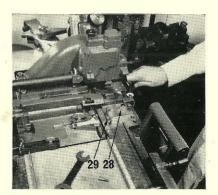
12. Place the mould blade slide in the forward position and attach to it the mould blade fork correct for the required point size.
