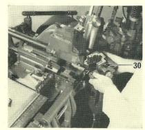
11. Attach the display matrix bridge (30) to the mould and secure in position with the three hexagonal screws.
