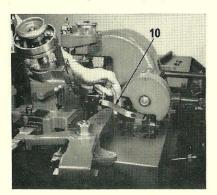
5. Unhook the actuating lever link (10) from the fusing stop on the mould and disconnect the elongated eye from the pin on the actuating lever. Remove the link from the machine.
