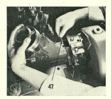
15. The mould blade slide driving block cap abutment must be positioned so that the large diameter end is toward the rear. Remove the end screw to reverse the abutment if necessary.
