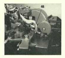
14. The actuating lever link (46) must now be attached. Slip the elongated eye over the actuating lever pin, and drop the hooked end over the fusing stop at the rear of the mould.
