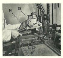
6. Remove three screws, and free the fourth screw (14), securing the display head (15). Take a firm hold on the head and lift it off.
