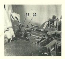
12. Connect the matrix lifter lever connecting rod eye (32) to the upper of the two holes in the matrix cam lever (33), with the eye pin and nut.
