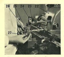
9. Assemble the counter bracket (22) to the main stand, locating the keys in the keyways, and securing with the four screws.
