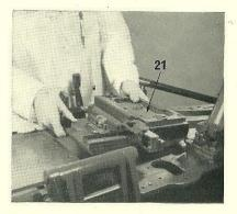
8. Disconnect the type pusher lever from the cam lever, by removing the nut and freeing the stud from the eye.
