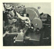
14. Attach the actuating lever link (37) by placing the elongated eye over the pin on the actuating lever, and hooking the other end to the fusing stop on the mould.
