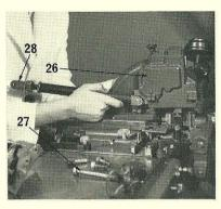
10. Place the display matrix head (26) in position on the matrix heads base.
