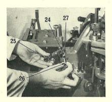
9. Place the mould blade slide (24) in the forward position and connect to it the mould blade fork (25). The connecting pin (26) should be inserted with a clockwise twist until it is just gripped in the yoke of the mould blade slide; in this position, tighten the small set screw (27) to retain it in place.
