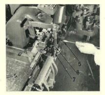
3. Remove the screw securing the water supply piping (5) to the mould, and remove the nut and washer securing the other end of the piping to the main stand stud. Take off the piping.
