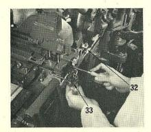
13. Cover the locating faces of the mould water supply piping (32) with grease, and fit over the stud on the main stand. Tighten the screw into the mould, and then tighten the nut and washer on the main stand stud.
