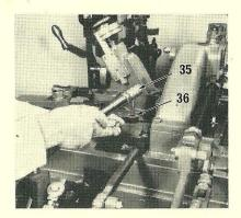
14. Connect the mould blade slide drive lever connecting tube ball end (35) to the required hole on the intermediate lever (36) making sure that the snug pin is seated in the groove before securing with the nut.
