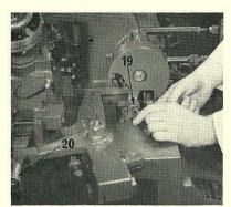
6. Detach the weight from the ratchet pin chain, and disconnect the actuating rod eye (19) from the actuating lever by removing the pin. Use the same pin to connect the lower hole of the rod eye to the actuating rod housing.
