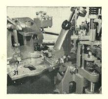
12. Bring the jet block driving rod forward so that its hook (31) is clear of the counter bracket. This will make it easier to locate the hook on the jet block in position over the hook on the driving rod when the mould is assembled on the machine.
