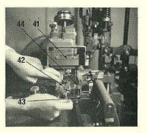
16. Attach the display mould guard (41) to the matrix head cover by inserting the hinge pin through the hinges.
