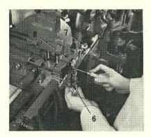
3. Take off the air nozzle and holder, and the cutter blade bracket. Remove the mould oiler (6), and disconnect the mould water supply piping (7). Take out the three screws which secure the bridge (8), and lift it off.
