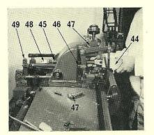
14. When continuous borders and dashes are to be produced, assemble to the counter bracket the continuous border matrix lifter (44). Slide the spring box (45) through the gap alongside the lead clamp intermediate lever spring box (46). Fit the key on the matrix lifter into the keyway on the counter bracket, press the matrix lifter bracket firmly against the stop, and secure in place with the bracket screw (47). Connect the spring box yoke (48) to the upper hole of the matrix cam lever (49).
