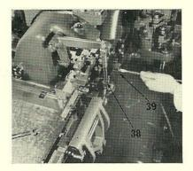
15. Connect the lead clamp intermediate lever rod yoke (38) to the lead clamp lever, unclipping the pin to make the connection, and re-clipping after having done so.
