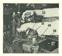
16. Position the cap abutment (47) with the large diameter end to the rear. and connect the spring plate by its upper hole to the spring post. Turn the eccentric fulcrum pin (48) to the 1-3 L and R position.
