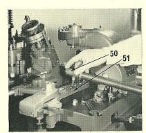
15. Connect the spring plate by the upper of the two holes to the swing frame post. Connect the mould blade slide drive lever connecting tube ball end (50) to the hole marked *Leads* on the intermediate lever (51).
