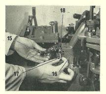
7. Assemble the mould blade fork (15), of the point size required in the following manner. Place the mould blade slide (16) in the forward position, and connect it to the fork with the pin (17), which should be inserted and turned clockwise until it is felt to grip. At this point, tighten the set screw (18).
