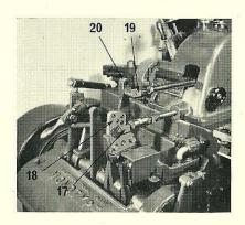
7. Disconnect the jet block driving rod connecting rod yoke (17) from the type carrier cam lever extension (18) by removing the screw and the yoke position pin.
