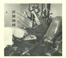
15. Place the stop lever handle (37) in the uppermost position. Turn the eccentric fulcrum pin to indicate the required point size of type. Check that the driving block cap abutment is set for the set size of type to be cast, i.e. for set sizes above 12 point the large diameter end should be towards the rear of the machine.
