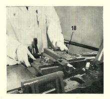
9. Place the matrix heads base (18) in position on the main stand, locating the keys in the keyways. Check that the base locating key distance piece is in the required point size position, and reverse if necessary.
