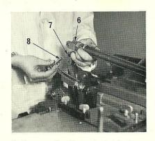
3. Remove the air nozzle holder from the cutter blade bracket; the matrix holder from the Display matrix head; and the matrix lifter lock wedge spring box voke (6) from the matrix cam lever (7), by removing the connecting pin (8).
