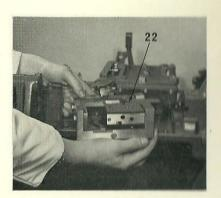
8. Turn the machine to 220°, and remove the three screws from the mould base. Remove the clamps from the front and side of the mould.
