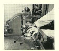
6. Turn the machine to 200° and pull back the fusing stop to place the mould blade slide in the forward position. Disconnect the mould blade from the slide by releasing the set screw and removing the pin. Re-tighten the set screw.
