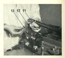
4. Disconnect the matrix lifter lock wedge spring box yoke (11) from the matrix cam lever (12) by removing the pin (13).
