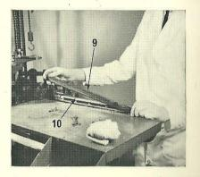
4. Remove the two screws and washers securing the lead stacker bar (9) to the lead stacker (10), and lift it off. The lead stacker bar does not need to be taken off the machine except for the production of Furniture.
