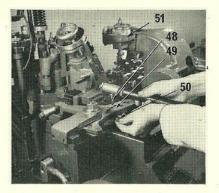
16. Connect the mould blade slide drive lever connecting tube ball end (48) to the hole marked *Furniture* on the intermediate lever (49), seating the snug pin into the groove and securing with the nut (50).
