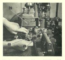
16. Attach the mould guard (39) to the matrix head cover by means of the hinge pin. Place a matrix into the matrix holder, and insert the holder (40) into the matrix lifter. Attach the cutter blade bracket (41), locating its key into the keyway on the main stand, and securing with the washer and long screw through the front locating hole. Assemble to the bracket the air nozzle holder and air nozzle.
