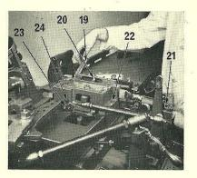
8. Substitute, if necessary, the fixed type channel block (19) for a block suitable for the product to be cast.
