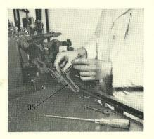
12. Fit the furniture guide (35) to the main stand, using the cutter blade bracket screw, the collar, long screw and washer. Release the lead clamp and insert a piece of product of the required size into the mould.
