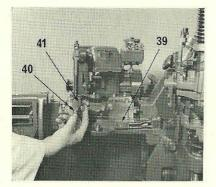
14. Attach the mould water supply piping (39) marked LR and Furniture; grease the locating faces, and secure to the mould with the screw and, to the main stand stud with the nut and washer.
