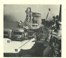
5. Release the nuts (9) on the mould blade fork and, with the aid of a pin handle (10), remove the fork pin, disengaging the fork from the mould.
