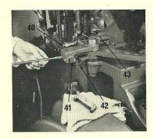
13. Check that the mould blade slide driving block cap abutment (40) is correctly positioned, and reverse if necessary. For set sizes 12 point and below, the end having the large diameter should be towards the front.
