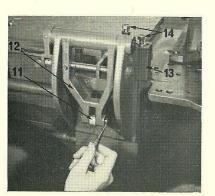
5. Disconnect the cutter actuating plunger link (11) from the cutter actuating lever (12) by removing first the split pin and then the cutter actuating pin.
