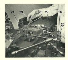
9. Connect the type carrier connecting rod yoke (25) to the hole on the cam lever extension (26) marked 12 for small type, or 24 for large type, using the pin and split pin.
