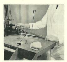
10. Attach the lead stacker bar (27) to the lead stacker (28) with the two screws and washers.
