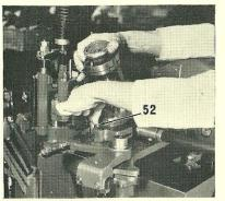
16. Use a 6-em border length gauge (52) as shown between the abutment plate and the mould blade stop; screw the wedge down until the gauge fits without binding; turn the scale to zero, and lock.
