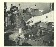
3. Disconnect the mould blade slide drive lever connecting tube ball end (6), from the intermediate lever (7), by removing the nut (8) and lifting the ball end free. Replace the nut onto the ball end and swing the tube clear of the intermediate lever.
