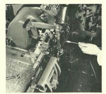
15. Grease the locating faces of the mould water supply piping, and with one end on the main stand stud, swing into place and finger tighten the nut (40). Screw into the mould, and then further tighten the nut with a wrench.
