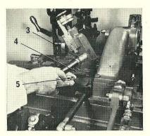
2. Disconnect the mould blade slide drive lever connecting tube ball end (3) from the intermediate lever (4), by removing the lock nut (5) from the ball end and lifting clear.
