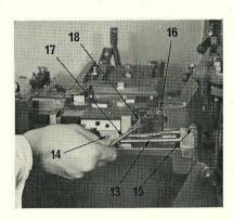
6. Disconnect the mould water supply piping (13), by removing the screw (14) into the mould, and the nut and washer (15) from the stud on the main stand. Take off the piping and replace the nut and washer on the stud. Slacken off the knurled lock nut and the knurled nut on the mould blade fork (16), and with the aid of a pin handle (17), remove the fork pin (18).
