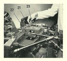
8. Lift off the counter bracket after removing the four screws, and in its place put the matrix heads base (21), locating the keys in the keyways. Check that the locating key distance piece (22) is facing correctly for the point size of type to be cast, then secure the base in position with three of the four screws; the remaining long screw will be used when the matrix head is assembled.
