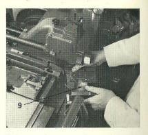
4. Loosen the nuts on the mould blade fork, and using a pin handle, withdraw the fork pin.
