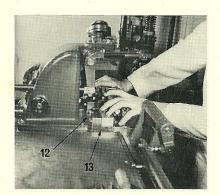
5. Turn the machine to 200° and pull back the fusing stop to place the mould blade slide in the forward position. Remove the pin connecting the mould blade to the mould blade slide, and disconnect the actuating lever link. Take out the screws securing the mould to the main stand, and remove the clamps. Push the jet block a little way out of the mould to provide a clearance, disengage the hooks (12), and remove the mould (13).
