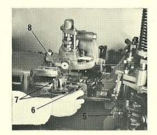
3. Remove the air nozzle and holder; the crossblock oiler, and the mould oiler. Disconnect the mould water supply piping (5), and after releasing the knurled lock nuts remove the mould blade fork pin with a pin handle (6).
