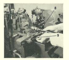
3. Disconnect the mould blade slide drive lever connecting tube ball end (7) from the intermediate lever (8), by removing the nut (9) from the ball end. and lifting the tube clear. Replace the nut on the ball end, after removal of the tube, to avoid losing it.
