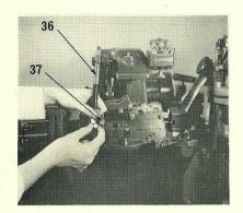
13. Re-connect the lead clamp intermediate lever rod (36) to the mould with the yoke pin. Make sure that the clip (37) is pressed back over the pin to hold it in place.
