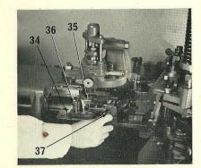
13. Assemble to the mould adaptor base first, the type clamp operating block, and then the composition mould, locating with the knurled screw (34) and securing with the base screw.
