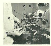
11. Place the counter mechanism head (28) in position on the main stand, and secure with its four screws (29). Connect the lead clamp intermediate lever (30) to the lower hole in the matrix cam lever (31), and the position pin on the jet block driving rod yöke (32) to the 12/12 position on the type carrier cam lever extension (33). Insert the yoke position pin screw to secure the pin in its location.
