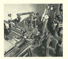
14. Grease the locating faces of the mould water supply piping (41) marked 'A.B.' and attach to the main stand stud. Screw the piping to the mould and then affix the washer and nut to the main stand stud.
