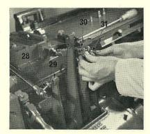
10. Connect the type pusher lever connecting rod ball stud (28) to the type pusher cam lever (29), securing with the nut.
