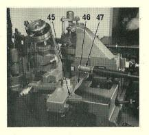
16. Set the eccentric lever fulcrum pin (45) on the mould blade slide drive lever (46) to the required position marked 5—36 type.
