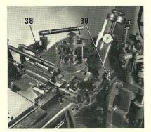
14. The type support spring cam bracket (38) should be used to produce all type up to 36-point body size and not more than 12-point set size.
