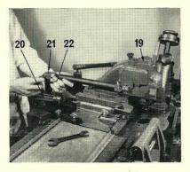
10. Assemble the display matrix head (19) to the matrix heads base, securing with the three screws and also the long screw into the main stand.
