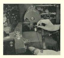
6. Since the counter mechanism will not be required for production of display material, the counter bracket will need to be removed.
