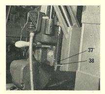
15. Connect the lower pump body lifting spring plate (37) by the upper one of its two holes to the swing frame spring post (38).
