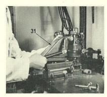
11. Assemble the composition matrix head (31) on the matrix heads base, locating the keyways over the keys on the base. Secure in position with the one long screw and the three shorter screws.
