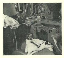
11. Pull the intermediate lever (35) to the left to disconnect it from the plate (36), and then change the plate for the one marked *Furniture* by removing the two screws.
