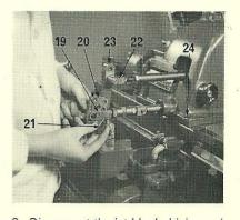
8. Disconnect the jet block driving rod connecting rod yoke (19) from the cam lever extension (20) by removing the screw and position pin (21).
