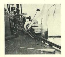
13. Attach the furniture guide (36) to the main stand with the long screw, washer and collar from the cutter blade bracket
