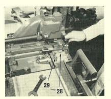
10. With the machine set at 220° and the micrometer wedge indicating a mould opening of 60 point, attach the mould (28) to the main stand by sliding the type carrier hook into engagement, and then locating it against the matrix heads base. Secure to the main stand with the clamps (29) at the side and front, and the three mould screws underneath.
