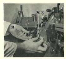
10. With the mould blade slide (30) in the forward position, attach to it the appropriate mould blade fork (31). Insert the connecting pin, and twist until it is felt to grip; at this point, tighten the set screw (32).
