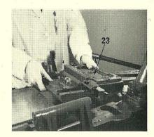
8. Place the matrix heads base (23) in position on the main stand, locating the keys in the keyways. Check that the locating key distance piece (24) (see picture 9) is in the correct position for 5—36 point. Secure the matrix heads base to the main stand using the three base screws.
