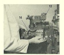
5. Place the oiler valve lifters (13) in the horizontal position, and disconnect the oiler piping and support. Turn the machine to 20° and remove the product from the mould. Raise the mould blade stop lever handle, and then pull the mould blade slide drive lever towards you. This will enable the pin to be removed, which will disconnect the mould blade slide from the mould blade.
