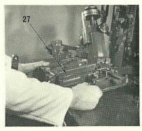
10. Take out the three screws which hold the matrix heads base to the main stand. Grasp the matrix heads base (27) firmly in both hands and lift it off, complete with the type pusher lever connecting rod and the type carrier connecting rod. Wipe the main stand
