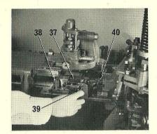
13. Attach either the large or the small composition mould and adaptor base assembly (37) to the main stand, engaging the mould coupling hook with the hook on the type carrier. Locate the adaptor base against the matrix heads base with the two clamps (38), and secure to the main stand by means of the long, medium, and short screws in their respective holes.
