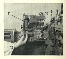
4. Disconnect the mould water supply piping by loosening the nut (9) on the main stand stud and withdrawing the screw (10) from the mould. Pivot the piping on the stud away from the mould so that it is ready for re-connection later.
