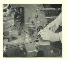
12. Connect the upper hole of the actuating rod eye to the actuating lever (38), using the pin previously removed.
