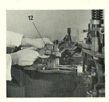
5. Take off the mould oiler, and then remove the three screws which secure the display matrix bridge. Having done this, lift off the bridge (12).
