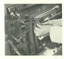
9. Remove the nut securing the type pusher lever connecting rod ball stud to the matrix cam lever, and disconnect the type pusher lever (23) from the cam lever (24). Replace the nut on the ball stud.
