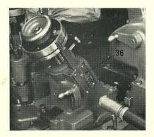
12. Position the mould on the adaptor base and secure it with the locating screw. Position the low quad lever for either high or low product, and connect the spring plate to the mould blade lever. Screw the type clamp operating block to the adaptor base.
