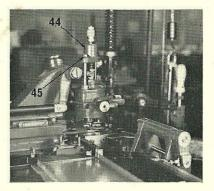
16. Sorts casting for large type composition will require the use of the centring pin auxiliary loading spring bridge (44) instead of the loading spring bridge normally in position on the composition matrix head.
