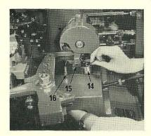
6. Unhook the weight (14) from the ratchet pin chain of the counter bracket. Disconnect the actuating rod eye from the actuating lever (15) by removing the pin (16). Re-connect the lower hole of the rod eye to the rod housing with the same pin. Loosen the machine.
