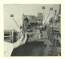
14. Grease the locating faces of the mould water supply piping (33) and connect to the mould with the screw. Tighten the nut on the main stand stud.
