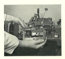
7. Turn the machine to 220°, remove the three screws from the mould base, and remove the clamps from the side and the front of the mould. Slide the mould (19) towards the melting pot to disengage the hook from the hook on the type carrier, and lift off the mould.
