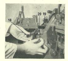
7. Disconnect the mould blade fork (18) from the mould blade slide (19) by slackening off the set screw (20) just sufficient to remove the connecting pin.
