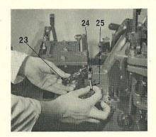
9. Substitute, if necessary, the mould blade fork (23) already connected for the one suitable for the product to be cast.
