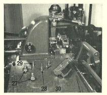
10. Secure the mould to the main stand with the clamps (27) at the front and side, and tighten so that it is brought firmly against the locating faces on the counter bracket and the wedge screw housing. Insert the four screws (28) into the top corners of the mould.
