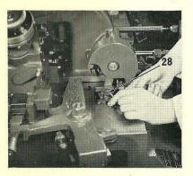
10. Disconnect the actuating rod eye from the rod housing by removing the pin. Use this pin to reconnect the upper eye of the rod (28) to the actuating lever.
