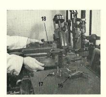
7. Loosen the thumb screw and remove the adjustable type channel block (16). Remove the three remaining screws (17) securing the matrix heads base (18) to the main stand, and lift the base clear of the machine.
