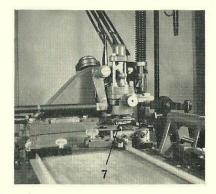
3. Remove the matrix holder (7) from the matrix lifter. Disconnect the air nozzle holder, air nozzle and collar, and the crossblock oiler from the main stand by removing the long screw and its washer.
