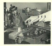
2. Disconnect the mould blade slide drive lever connecting tube ball end (3) from the intermediate lever (4) by removing the locking nut (5). Replace the nut on the ball end to avoid loss.
