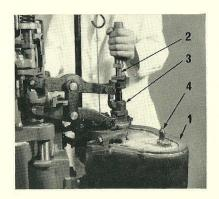
Changing from Sorts Casting for Small or Large Type Composition to Display Type Casting, Quotations or Wooden
