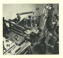
14. Close up the adjustable type channel block (44) to the fixed block (45), and secure to the type carrier cover with the screw and washer (46). Grease the locating faces of the mould water supply piping (47), and connect the piping to the mould. Attach the mould oiler to the mould (not shown), and insert the matrix holder complete with a matrix into the matrix lifter.
