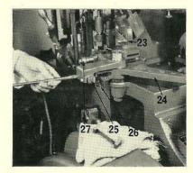
11. Place the stop lever handle (23) in the low position. Slacken off the spring adjusting nut. Set the fulcrum pin at the 1—3 L and R position.
