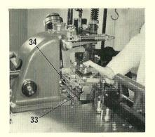
10. Place the mould (33) on the main stand, raising the back slightly so that the hook (34) on the jet block will engage the hook on the driving rod. Insert the clamps at the front and side of the mould, tightening until it is brought into correct location against the faces of the counter bracket and the wedge screw housing. Secure to the main stand with the four screws.
