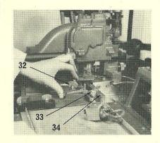
13. Loosen the thumbscrew (32) on the adjustable type channel block and insert a piece of product (33) to set it for size. Having adjusted the block, tighten the screw again. Note: When casting over 84 point set size, remove the fixed type channel block (34).
