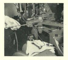
8. Place the lead mould blade stop lever handle (17) in the position marked *Leads*. Turn the adjusting nut anticlockwise so that minimum spring pressure is exerted. Set the fulcrum pin at the 1—3 L and R position. Disconnect the intermediate lever (18) from the plate by pulling it towards the cams.
