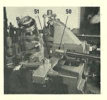
16. Connect the mould blade slide drive lever connecting tube ball end (50) to the hole marked *Type to 42* point on the intermediate lever (51), making certain the snug pin seats into the groove. Lock in position with the nut previously retained on the ball end.
