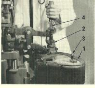
1. Switch off the electric motor; turn off the water supply; and place the gear control in the neutral position. Lower the melting pot (1) and, if necessary, change the pump body (2), nozzle (3), and piston (4) so that they will be at the correct temperature for casting when the change-over has been completed.
