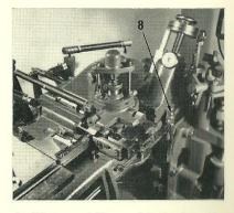
4. Disconnect the mould oiler from the mould; and also the water supply piping (8) which is held by a screw into the mould and a nut and washer on the main stand stud.
