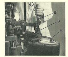
2. Fit the pump (3), nozzle (4) and piston (5) required for the change of product, so that the parts have time to attain the working temperature whilst the change-over is being made.
