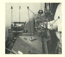
3. Remove the continuous border matrix lifter (6) from the machine, if attached, in the following manner.
