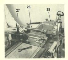
9. Assemble the Display matrix head (25) to the matrix heads base, locating the keyways on the head over the keys on the base. Secure with the four screws.
