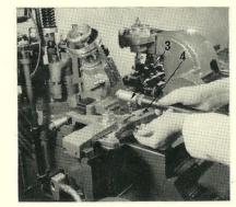
2. Remove the mould oiler piping and support from the underside of the mould oiler by releasing the knurled nut.
