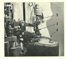
2. Fit the pump (3), nozzle (4) and piston (5) required for the change of product, so that the parts have time to attain the working temperature whilst the change-over is being made.
