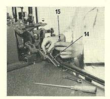
6. Remove the furniture guide (14) from the main stand, by releasing the cutter blade bracket screw (15) which has been used to secure it in position.
