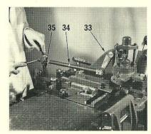
11. Assemble the composition matrix head (33) on the matrix heads base, and secure it in place with the three short screws and one long screw.
