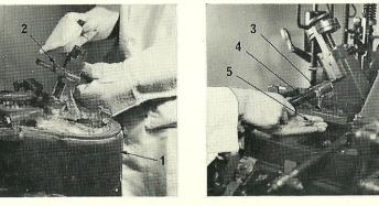
2. Disconnect the Mould Blade slide drive lever connecting tube ball end (3) from the intermediate lever (4), by removing the nut (5) from the ball end and lifting the tube clear. Replace the nut onto the ball stud to avoid loss.
