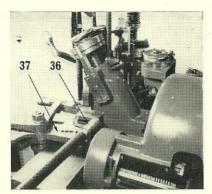
15. Connect the mould blade slide drive lever connecting tube ball end (36) to the hole marked *Leads* on the intermediate lever (37); seat the snug pin into the groove and secure with the nut.
