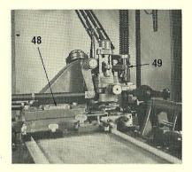
15. Attach the type support spring cam bracket (48) to the matrix heads base for type up to 12 point set size, and add also the packing plate for type over 36 point body size. Remove the upper and lower plates (49), and lift up the nozzle seating device to place it out of action. Connect the pump body lifting spring plate to the spring post by the lower hole for small type, or the upper hole for large type.
