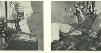
2. Disconnect the mould blade slide drive lever connecting tube ball end (5) from the intermediate lever (6), by removing the nut (7) from the ball end and lifting the tube clear.
