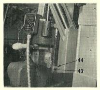
15. Attach the mould oiler to the mould, and then connect the pump body lifting spring plate (43) to the swing frame post (44) by its lower hole for small type, or the upper hole for large type.
