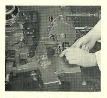
7. Remove the pin to disconnect the actuating rod eye from the actuating lever (18). Connect the rod by the lower of the two holes to the rod housing, using the same pin as before.
