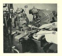
16. Connect the lower pump body lifting spring plate by the upper hole to the swing frame post.
