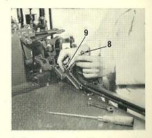
4. Remove the product from the mould, and take out the cutter blade bracket screw (8) holding the furniture guide (9) in place. Take off the furniture guide.
