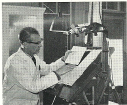
ABOVE Four butt-joint plates being loaded into the vacuum copyholder of a fixed-focus camera.
