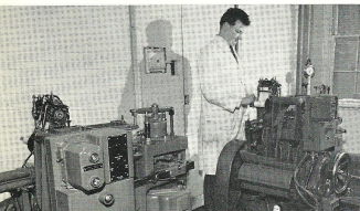
BELOW For calculating the acreages (to two decimal places) of land parcels for insertion on the 1/2500 plans, an Automatic Reading Planimeter is used.
