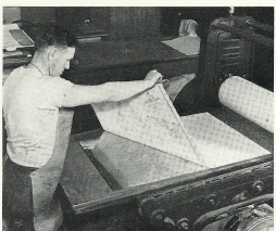
Taking a proof from a copper plate.
