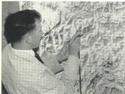
BELOW: Hillshading being produced with an air brush at the Small Scales Division of the Ordnance Survey.
