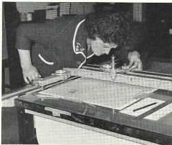
BELOW Plotting control points on field documents with a co-ordinograph, the permanent ones being enclosed by yellow symbols and the non-permanent ones by blue symbols.
