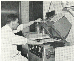
ABOVE An electronic contact box for producing photographic prints. This device, fitted with scanning apparatus, prevents any cloud shadow on a negative from obscuring ground detail on a subsequent print.
