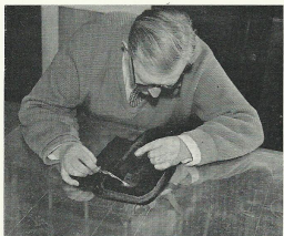
Local etching of chart detail into a copper plate.
