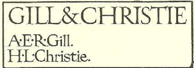
Fig. 2: From a drawing 1"×4", dated May 17th, 1907, and inscribed in Gill's hand "Name plate to be etched in white metal and letters filled in with Blackwax" and "N.B. No reduction".
