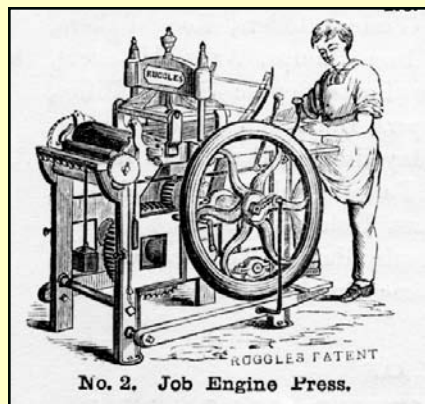
Left, Ruggles' "Upside-down Press" of 1840; right, his Rotary Job Press of 1849—the direct antecedent of the modern platen job press.
