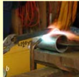
(a–d) heating and bending 1" solid bar over a section of pipe to achieve the desired curve for the stop (e) drilling one end for a bolt
