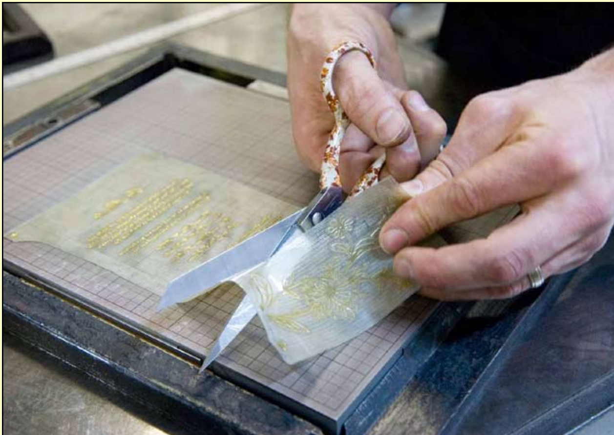
Boxcar Press sells plastic-backed photopolymer plates that are easily cut with scissors.
