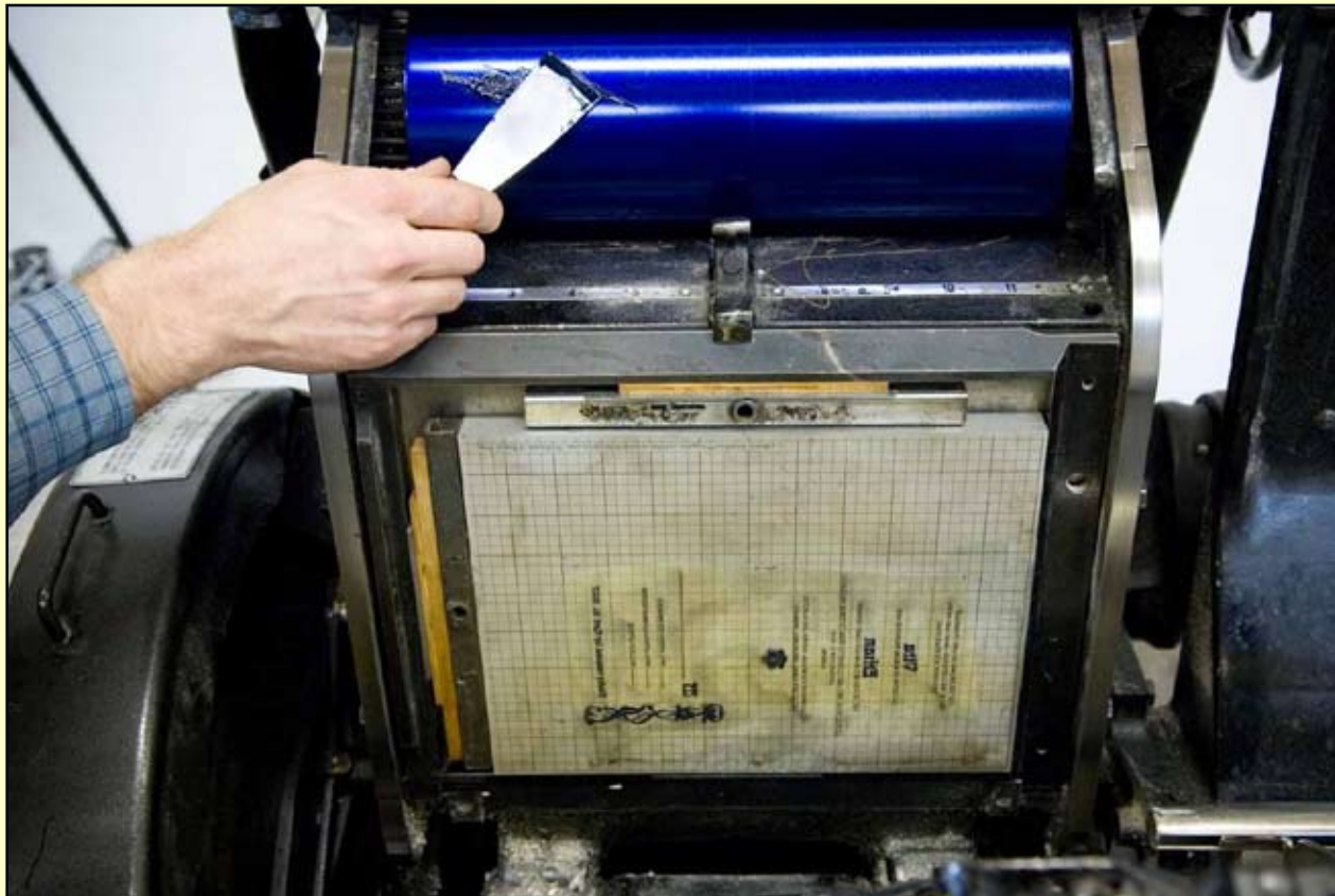
Inking the 10x15 Heidelberg Windmill locked up with a 9"x12" Standard Boxcar Base and KF95 plates.
