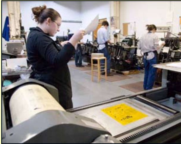
All plates made for Boxcar Press's platemaking customers are tested on a Vandercook Universal III before quality inspection by two different employees.
