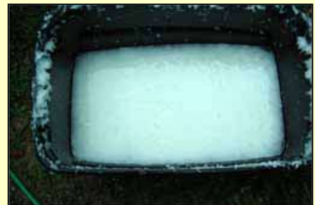
The partially beaten Half-Stuff in the tub is the results of around ten minutes of beating with the paint stirrer and electric drill. To reduce the pulp to a useable fineness another 20 minutes or so of beating will be needed.
