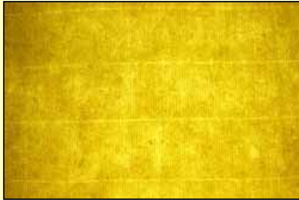
The clear chain and laid lines of a modern laid mould can be seen in this photo of a finished sheet.
