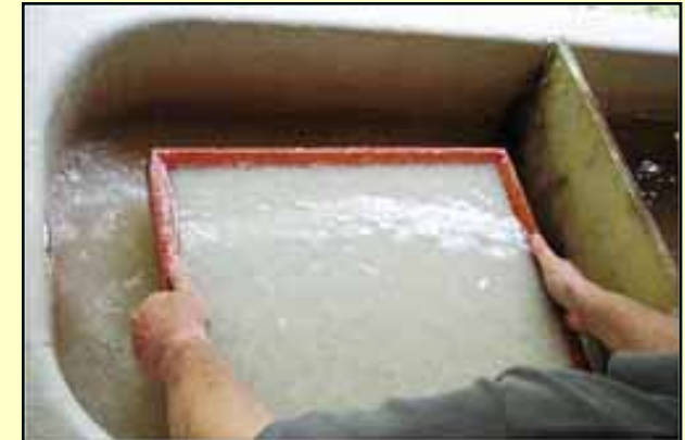
The wave can be clearly seen in this photo. As the wave reaches the top of the mould the slight shaking left, right, forward and back will begin.
