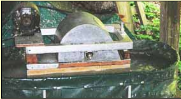
The Hollander with roller down and splash guard cover in place.
