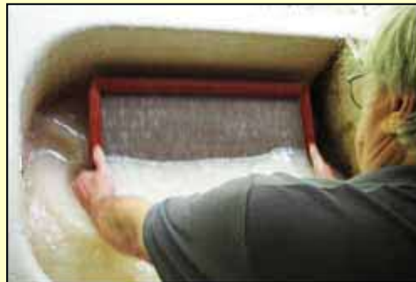
The tub has been stirred by hand to get the stuff mixed with the water. The mould is extended across the tub and submerged about 2/3rds of the way into the vat, then slowly lowered completely into the tub while being moved back toward the caster.
