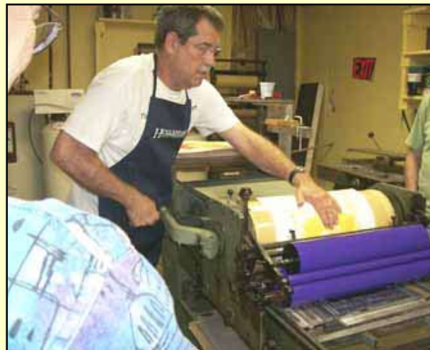
Jim is now rolling the sheet over the form. The rollers are not inking at this point.
