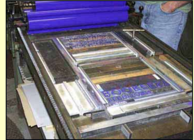
Here is the type in the form, set up after the Ginkgo branch and leaf images have already been printed.
