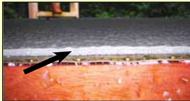
The thin layer of pulp (approximately 1/8-inch) can be seen in this close up of the mould with the deckle removed.
