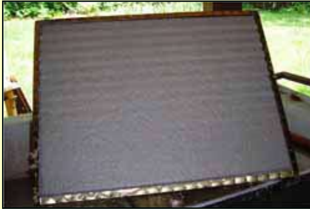
The ribs of the mould can be seen through this newly cast 15 x 19-inch sheet resting against the asp while it drains.
