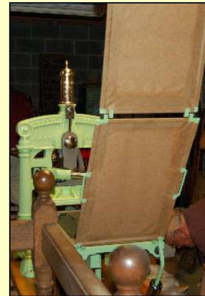
The Albion with tympan and frisket attached.
