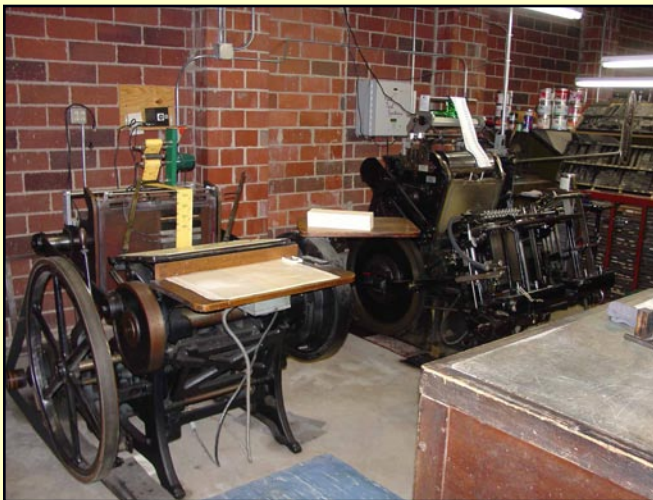
A 14x22 C & P handfed and a 13x18 Heidelberg platen have been fitted with foiling stamping units, and provide a specialty niche for the company.
