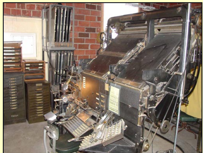
One of five Intertypes in the hot metal composing room is this G-4-4 Mixer, which was built to set complex grocery ad type.
