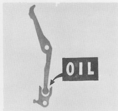
Illustration #11A. Where to Oil Escape Levers on Late Style Models 5, 8 and 31 Linotypes.
