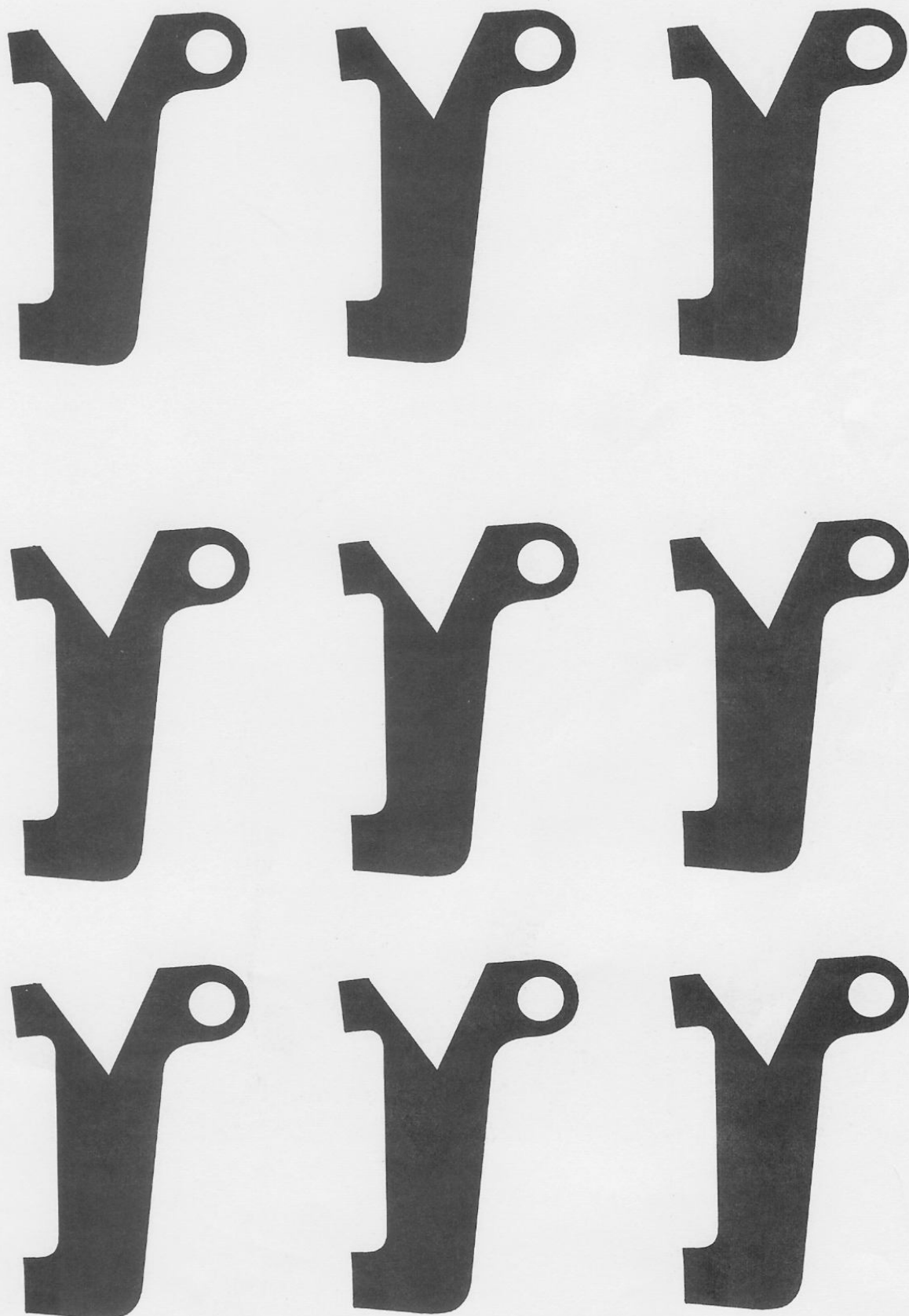
Illustration #37. Templates for Comet Assembling Cover Bracket, notching for light beam.
